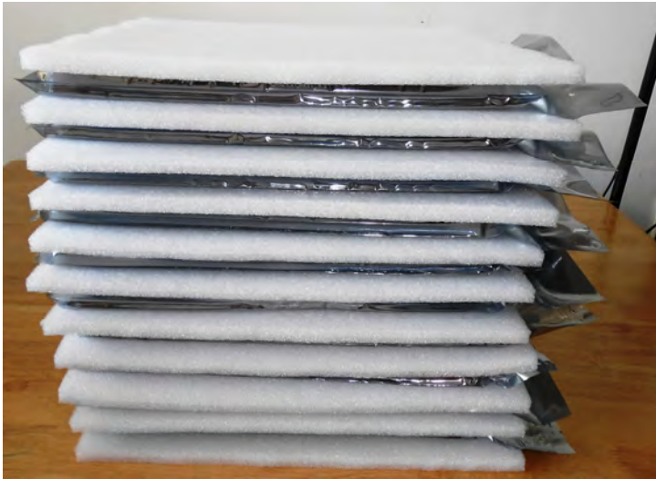
Place Foam Sheets Between Trays
